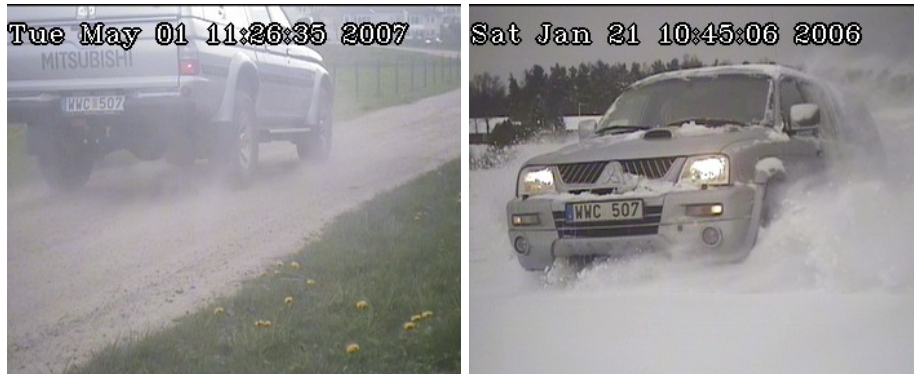
Figure 10: Dust and snow whirled up by a vehicle, obscuring its rear license plate.
