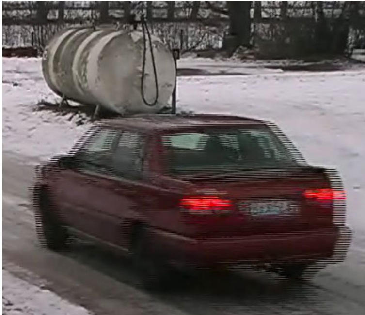
Figure 3: An example of the interlacing effect. Odd and even rows are not captured at the same time, there is a 20 millisecond offset between them causing objects in fast motion to appear garbled.
