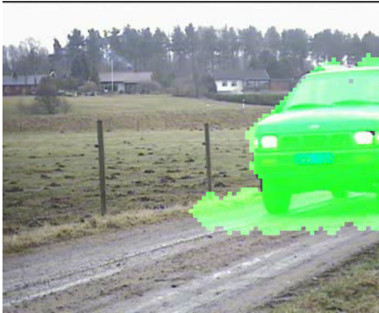
Figure 4: The marked area is classified as foreground by the simplified Stauffer-Grimson algorithm. Noise has been removed by morphological opening.
