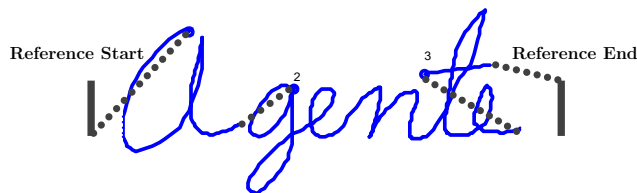
FIGURE 4.3: A cursive word sample plotted with virtual reference segments in solid bars before and after the words. The dotted lines mark the pen-up segments in the sample.
