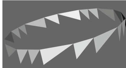
Fig. 2. The boundary and conormal constraints can be imposed by pre-specifying suitable triangles to be part of the surface
