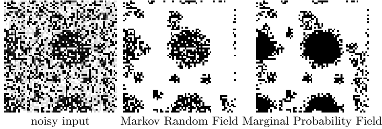
Fig. 3. Image denoising with MRFs and MPFs. We manually selected the best weighting parameter for each method. Both results are globally optimal.
