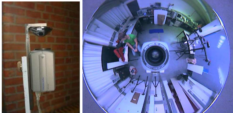
Figure 2: The camera setup and an image from the omnidirectional camera.
