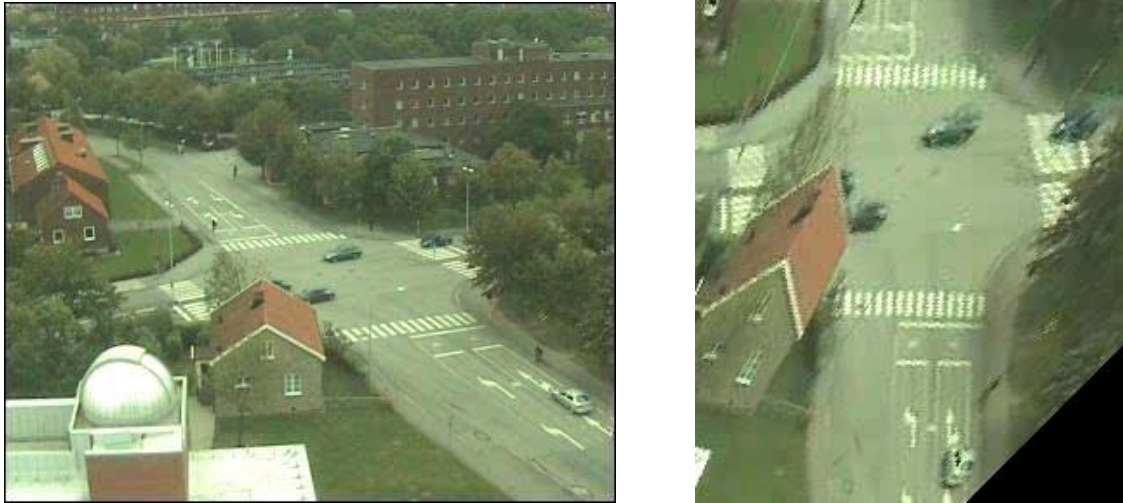
Figure 2. Rectification. To the left is the original image as produced by the camera and to the right is the same image rectified. Note that the road plane is rectified nicely while objects above the road get more and more distorted the higher they appear.
