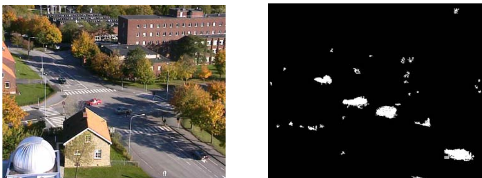
Figure 1. Foreground/background segmentation. To the left is the input image and to the right is the result after segmentation with the algorithm described in [17].
