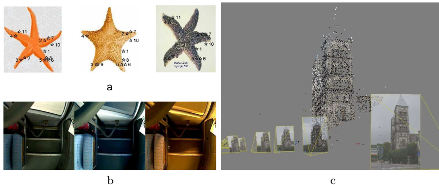
Fig. 1. Three methods of obtaining ground truth correspondences for vocabulary training using (a) deformable shape model (b) static scene with lighting changes and (c) structure from motion algorithms.
