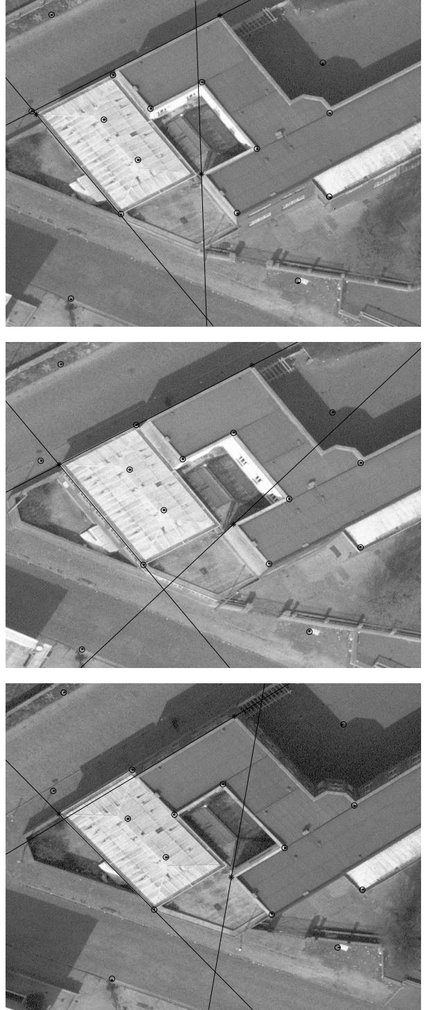
Figure 2: Three images with three extracted quivers shown in each image. Also shown are a number of points used to test the estimated solution. Original points are shown as '*' and reprojected points as 'o'.
