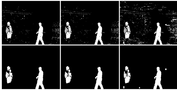
Figure 5. The result before and after morphological filtering for different thresholds, (Left) original result, (Middle) with 0.8, and (Right) with 0.4 threshold.
