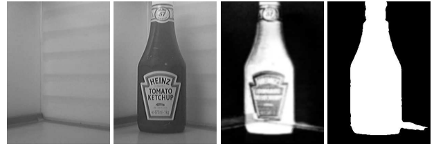
Figure 4: The two images to the left show the shelf before and after insertion of the object. The third image from the left shows the difference image. The rightmost image is a thresholded image.
