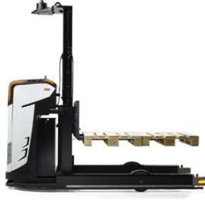
FIG. 1.1. An autonomous guided vehicle that uses one-dimensional vision to navigate.
