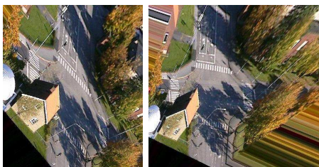
Figure 2: Output from the automatic rectification. To the left the algorithm worked on all tracks available. To the right some good tracks were manually chosen.
