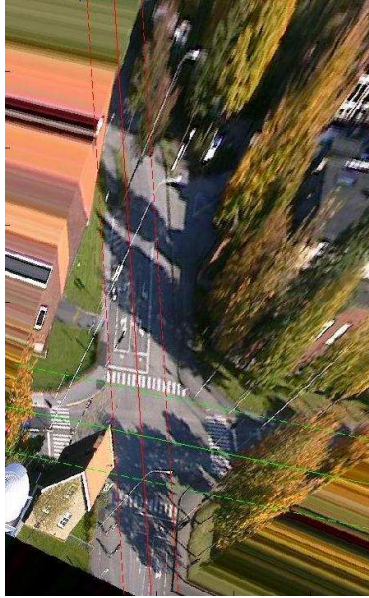
Fig. 3. The two roads in the image located approximately. Each road is represented by two lanes of opposite driving direction. The solid line shows the center of the road separating the two lanes and the two dashed lines shows the border of the road.
