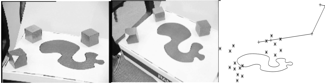
Figure 6: The Computer Vision Toolbox has been used to calculate the three-dimensional structure of the points and the curve, and the relative motion of the camera using the point and curve tracks.
