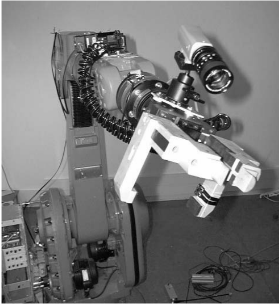
Figure 2.2: A robot with a hand-eye configuration.
