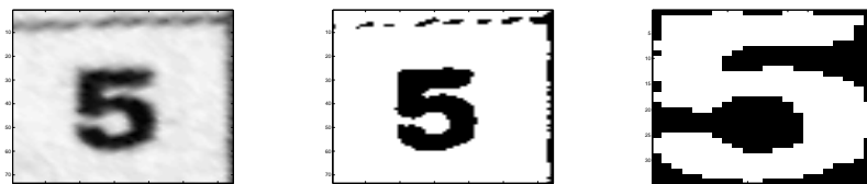
Figure 3: A cut out image of a digit is to be classified (left). First the image is normalized and thresholded (middle). Thereafter all connected components (of black) are found. The segment most likely to be a digit is selected (right).
