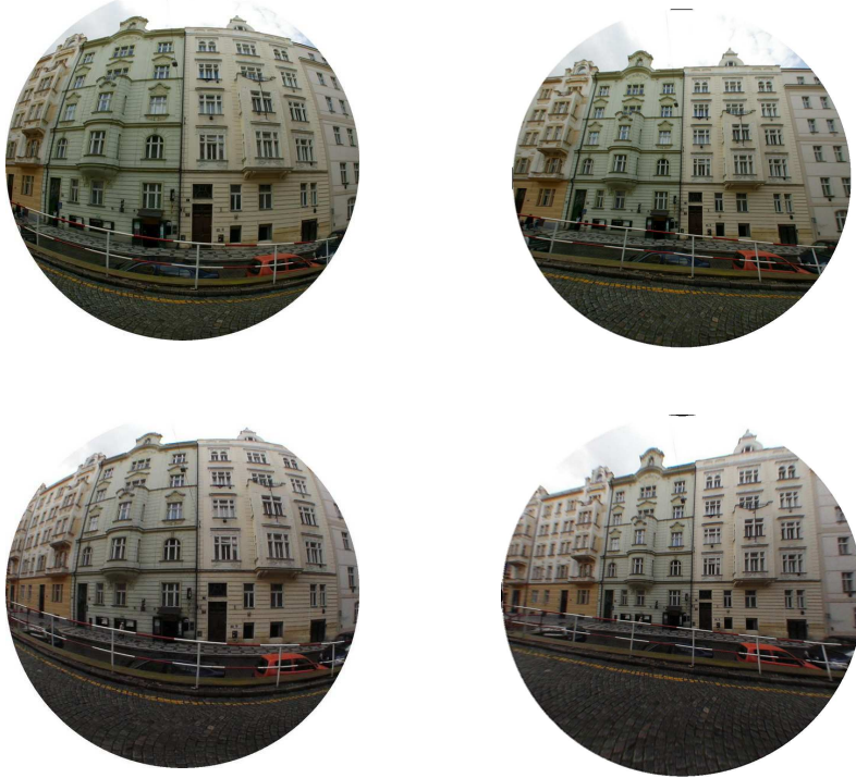
Figure 6.5: Real data, 60% cutouts from omnidirectional images. (Left) Input images with different radial distortions for camera 1 (Top) and camera 2 (Bottom). (Right) Corrected images.
